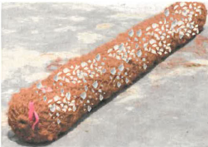
Experimental Ballasted Coir Using Native Shells. Images Camille Smokelin, Safe Harbor.
